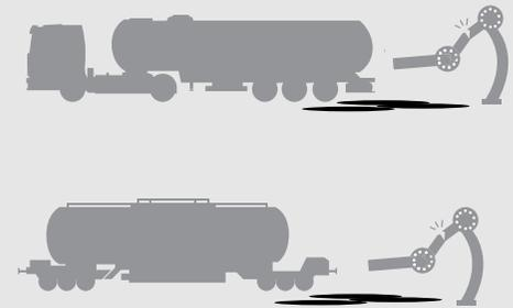
The lack of a Breakaway System in the event of a drive-off can be catastrophic.
